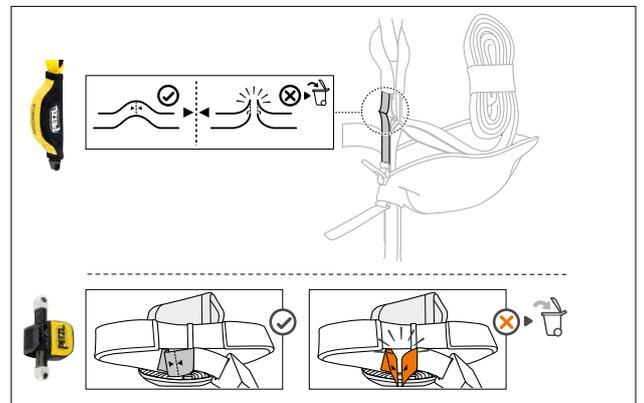
Verify that the energy absorber has not sustained an impact load (verify that none of the fabric between the straps has been torn).
